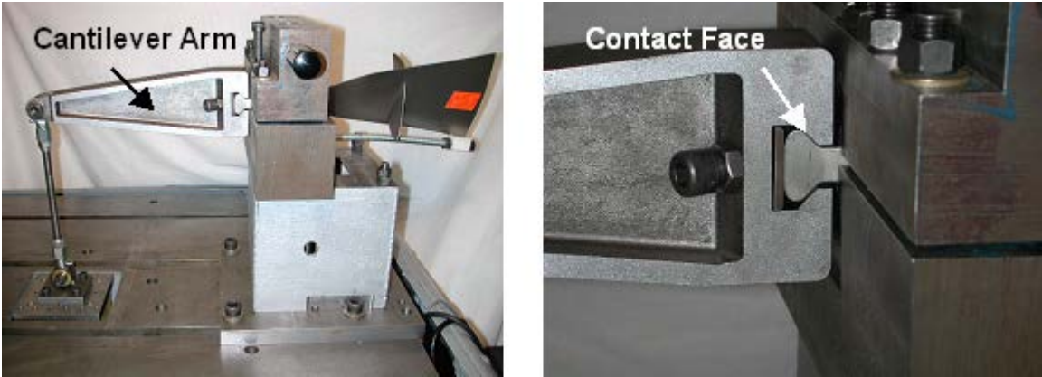
Figure 29 – Cantilever bending fatigue test set up for the F402 Stage 1 compressor blade.
