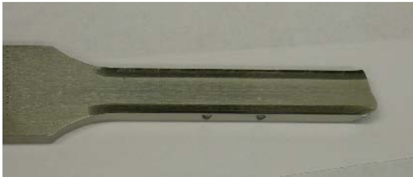
Figure 18 – A photograph of a LPB treated axial specimen. Notice the polished appearance of the specimen in the gage section. (Neu et al 2006 26 )
