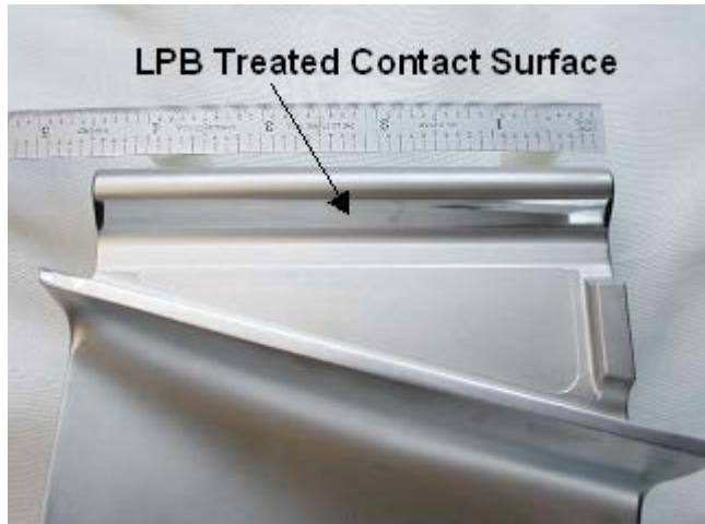
Figure 28 – LPB treated contact face of the dovetail in F402 Stage 1 compressor blade.
