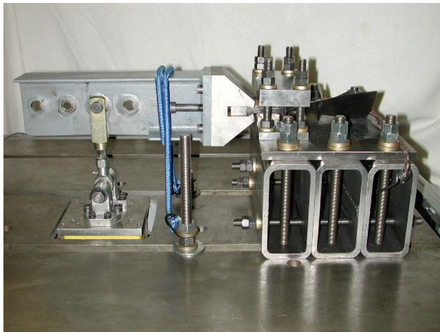
Figure 26 – Full scale fatigue test set up for the F404 Stage 1 compressor blade dovetail.
