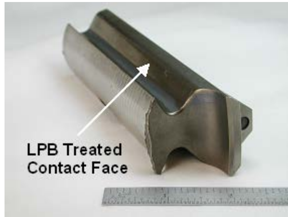
Figure 31 – An LPB treated disk post removed from the F402 Stage 1 rotor.
